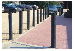
5. **Don't Rely on Car Stops or Curbs:** Standard 6 - 8 inch car stops or curbs are not effective barriers for moving vehicles. Once the wheels roll up over the edge, there's nothing to impede the vehicle's momentum.
