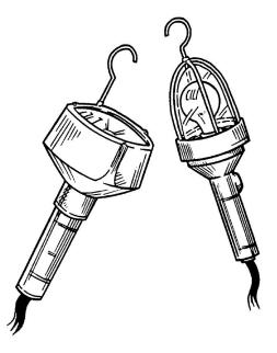
Portable lighting should be designed to eliminate ignition sources in the presence of flammable liquids or explosive atmospheres. Only lights tested and approved by recognized agencies such as UL, ULC, FM, NFPA, and Canadian Standards Association (CSA), shall be used with Class 1 Flammable liquids.
